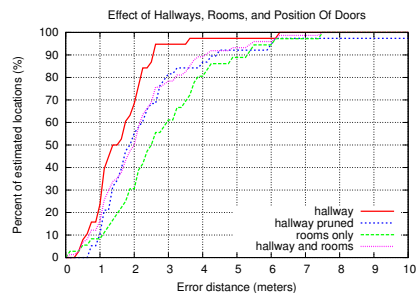
Fig. 12. The effects of hallways, rooms, and position of doors on location tracking accuracy. This data represents a limited data set in which the density of reference signatures in the hallway was pruned to match that of the in-room reference signatures.
